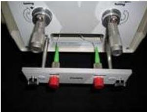
Easy access to optical connectors for cleaning. The connectors are located in a small drawer that can be opened for the cleaning operation.
