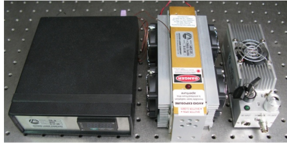
L: TC2 Temperature Controller M: L3S Laser R: RF Driver & Laser Controller
