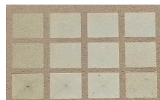
Surface burn-free marking on leather with fs-Green laser
