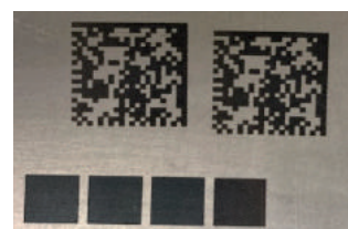
Anti-corrosion black marking on Ti with ps-IR laser
