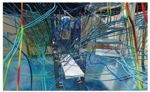
The sample illustration shows a CFD (Computational Fluid Dynamic) model of the air flow patterns in a typical OR.
