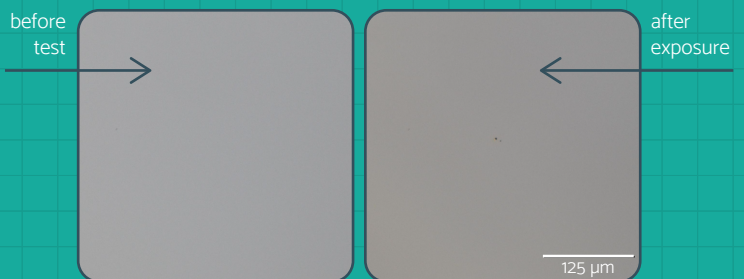
Typical damage morphology: fluence 4.39 J/cm 2 , damage after 100 000 pulse(s).
