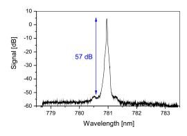
Typical Values: Power: > 1000 mW M<sup>2</sup> = 1.4 in both directions
