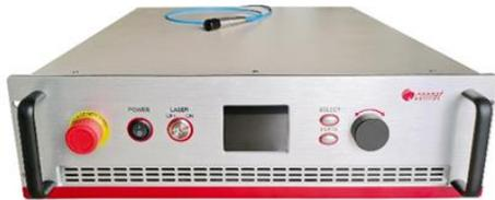
Based on the built-in 1018nm single frequency fiber laser, the 509nm single frequency fiber laser can achieve the real single frequency, single longitudinal mode and linear polarization output. The frequency doubling unit adopts the Periodically Polarized Lithium Niobate (PPLN) Technology. The 509nm laser maintains the low-noise performance of 1018nm single frequency fiber laser. The output power of the 509nm single frequency fiber laser can be up to 1W.
