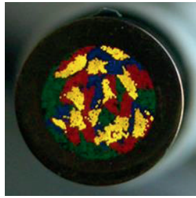
Coherent and randomized silica fiber bundle
