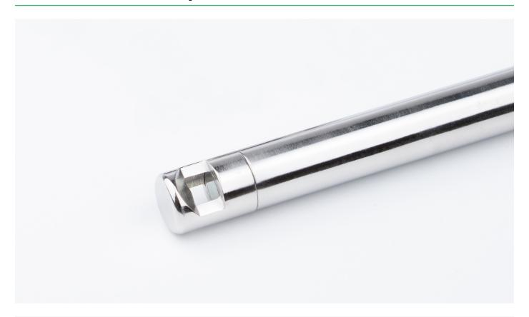
**FlexiSpec**® product line includes high sensitivity Transflection fiber optic probe to be used with any fiber optic spectrometer or photometer. They are available with a number of removable shaft heads, with slit width: 1, 2, or 5 mm (optical pass lengths 2, 4, 10 mm, respectively). These double-pass fiber probes have innovative collimated beam design, and bifurcated structure connecting the probe to both a light source and a spectrometer.
