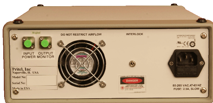
LNHP-PMFFA-xx model with Input/Output power monitor option
