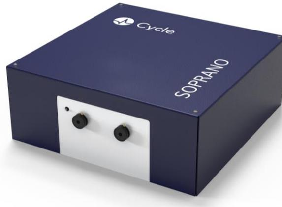
This femtosecond laser by Cycle is an ideal light source for various tasks in materials analysis and processing, semiconductor testing and more. With a center wavelength of 1550 nm and typically below 130fs pulse durations, many applications can benefit from this state-of-the-art ultrafast laser.
